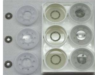
Figure 33. BioPress™ culture plate with acrylic pistons adhered to the silicone elastomer well bottom, foam sample holders (far left), and stationary platens (left of plate)
