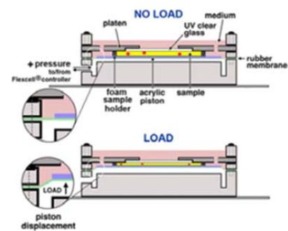
Figure 21. Compression application to cells in a StagePresser™ device
