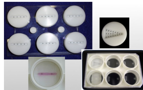
Figure 30. Representative image of 3D cell-seeded gel construct created in a Tissue Train® culture plate (left picture) and in a Trapezoidal TT® culture plate using a Trapezoidal Trough Loader™
