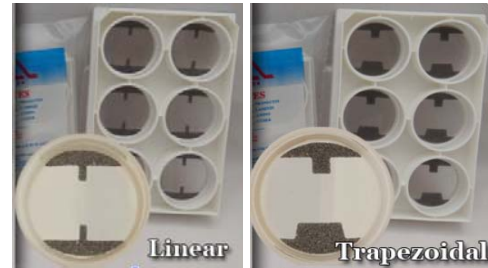
Figure 29. Tissue Train® and Trapezoidal Tissue Train® culture plates with the foam anchor stems
