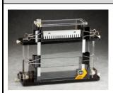
The JVD-80 Dual-Slab Vertical Gel System allows rapid analysis of protein and nucleic acid samples in a 16 x 18 cm polyacrylamide gel. This system allows analysis to be completed in less than 90 minutes while maintaining comparable resolution. For greater flexibility, the JVD-80 dual vertical system is adjustable from 16 cm to 42 cm or 62 cm thereby increasing resolution by 2.5x.
