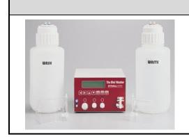
The IBI Blot Washer was designed to automate blotting procedures so they are performed exactly the same in order to eliminate the background. The Blot Washer is a programmable system that fully automates rinsing, incubating, and dispensing reagents needed for blotting procedures. It can even apply the secondary antibody.
